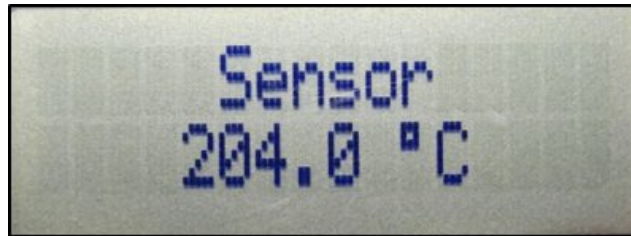
Figure 17 – Display with Process Variable Format
