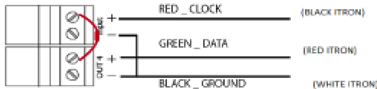
Figure 37: ORION Cellular LTE endpoint connection with resistor
